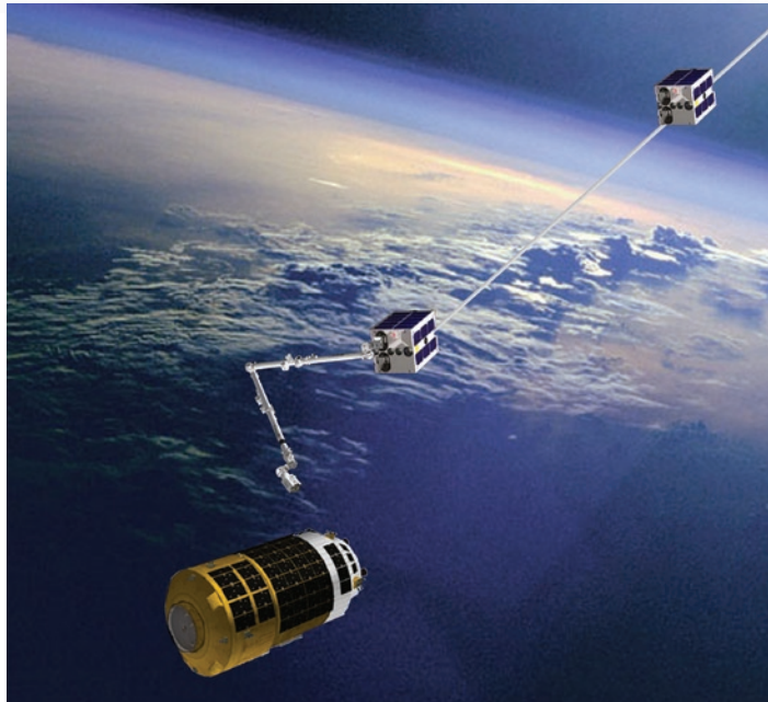
Figure 5. Most debris objects could be captured in nets, but some require a grappling device such as shown here. Devices like this have been developed and tested by NASA, DARPA, and the Naval Research Laboratory. (Canadian Space Agency, NASA, and wykesweb.com images)
