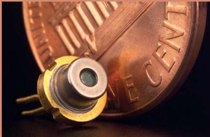
A 5.6 mm closed-can commercial laser diode, of the kind used for CD or DVD players. Photo: NASA
