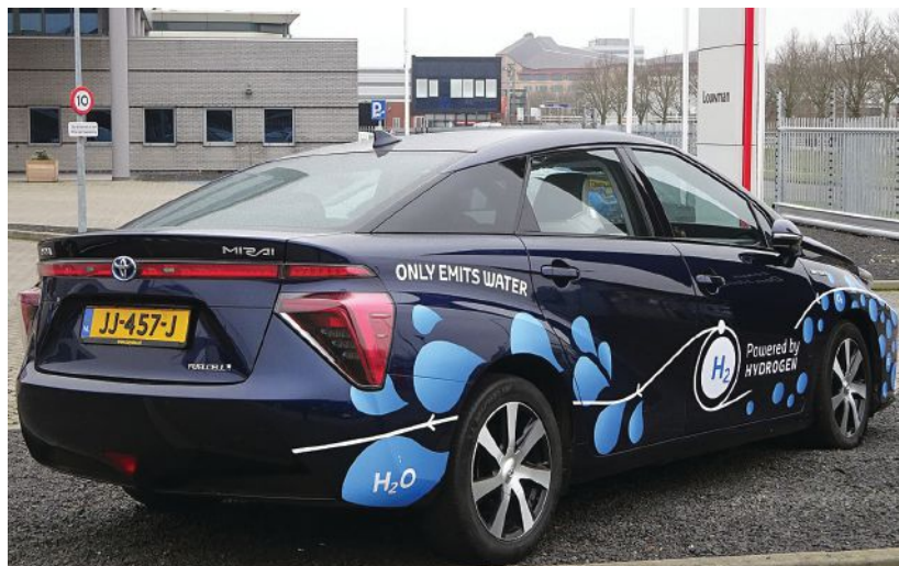
The 2016 Toyota Mirai, introduced in 2014, was the first hydrogen fuel cell car sold commercially. The car itself emits only water. However, hydrogen has to be produced and distributed for these cars. As there are a few hydrogen fuel stations at the moment in the Netherlands, the possible use of this technology is still limited. Credit flickr user harry_nl
