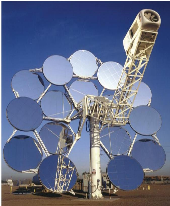
Mirrors in Arizona focus sunlight on a 25 kilowatt Stirling heat engine. Photo: U.S. Department of Energy
