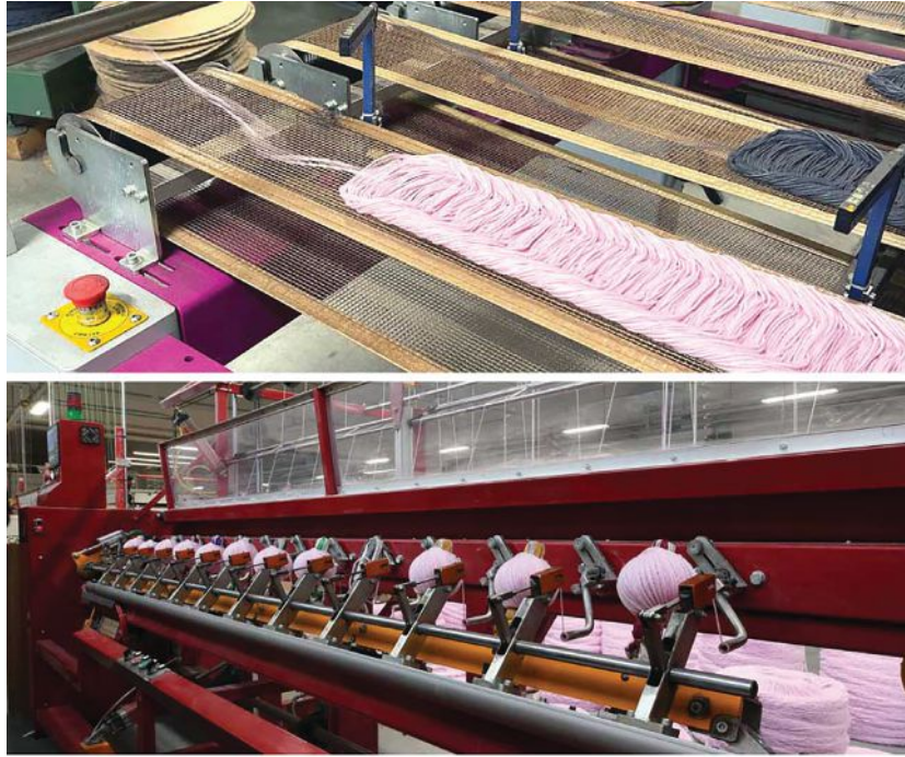
Figure 9: Yarn relaxing and balling. 7
