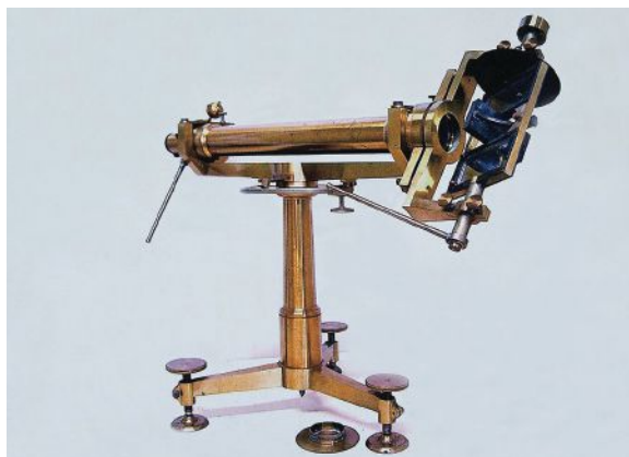
Invented in 1821 by Gauss, the heliotrope is an instrument that uses a mirror to reflect sunlight over great distances to mark the positions of participants in a land survey.
