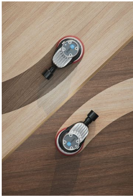
OnRobot has developed robot end-effectors, such as this sander, that are easy to swap and work with a variety of robot arms. Source: OnRobot
