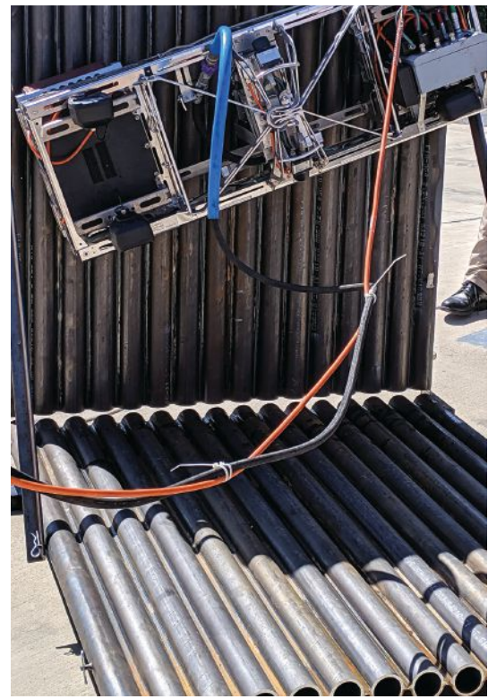
This maintenance robot from Baker Hughes inspects and cleans boiler waterwalls without requiring scaffolds or disassembly. Source: Baker Hughes
