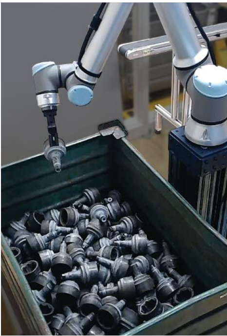
A Universal Robot cobot arm uses an ActiNav kit to pick unsorted parts from a bin. Source: Universal Robots
