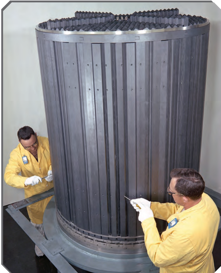
Figure 6: The MSRE core internal structure, assembled from individual extruded graphite components to form coolant channels on the perimeter of each piece. (ORNL Photo 70797)
