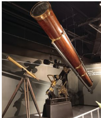
Figure 10: The Dearborn Observatory telescope, installed in 1866 at its first site in Chicago, was the largest refractor in the U.S. to have a wooden tube. The wooden tube was also used until 1911 at its second site on the campus of Northwestern University in Evanston. At that time, the objective lens was given a new steel tube and mount by Warner & Swasey. The wooden tube and its original brass mount by Alvan Clark & Sons have been preserved and are on display in the Adler Planetarium and Astronomical Museum in Chicago. Photo credit: Trudy E. Bell, June 2025.
