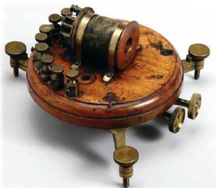
A mirror galvanometer is an ammeter that indicates it has sensed an electric current by deflecting a light beam with a mirror.
