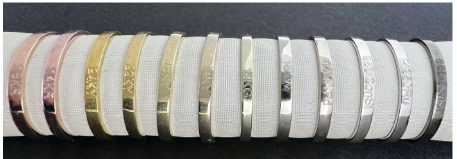
Figure 1: Different types and colors of metals. From left to right: 18K Rose Gold, 14K Rose Gold, 24K Yellow Gold, 22K Yellow Gold, 18K Yellow Gold, 14K Yellow Gold, 18K White Gold, 14K White Gold with Palladium, Continuum Sterling Silver, Platinum with Ruthenium, and Continuum Sterling Silver with Black Rhodium plating.
