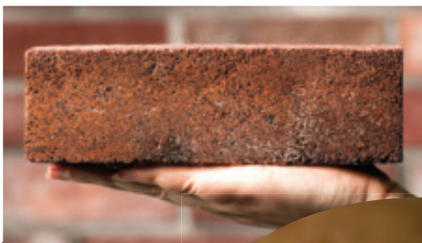
(Above) bioMASON makes bricks using only enzymes from natural bacteria. Image courtesy of bioMASON.
