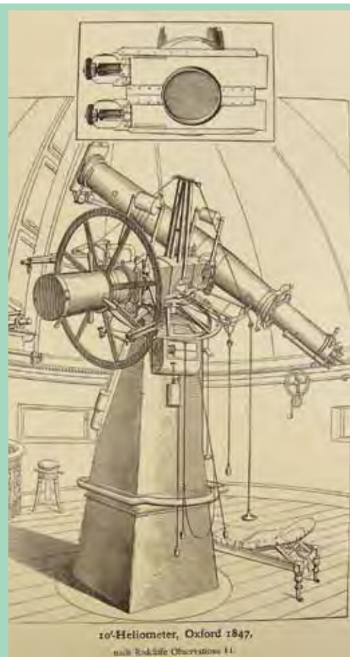
Fig. 4. The 7.5-inch heliometer at the Radcliffe Observatory at Oxford University, made by the Repsold brothers of Hamburg, was installed in 1848. Also called a divided-lens micrometer, its lens—like that of the Fraunhofer heliometer used by Friedrich Bessel at the Königsberg Observatory—was cut in half [inset at top], and one half slid away from the center of the other in order to measure small separations between celestial objects with great accuracy. [Credit: Joh. A. Repsold. Zur Geschichte der Astronomischen Messwerkzeuge von 1830 bis 1900 . Leipzig: Verlag von Emmanuel Reinicke, 1914.]
