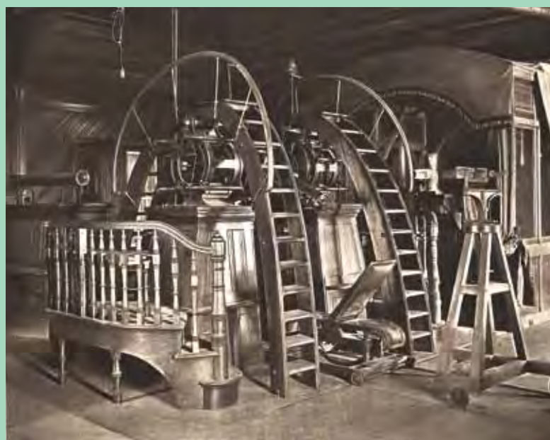
Fig. 1. This 6.4-inch meridian circle by the German instrument makers Adolf and Georg Repsold, installed at the Lick Observatory on Mount Hamilton, CA, in 1884, is almost unrecognizable as an astronomical instrument. The telescope, half-hidden near the center of the image above the half-reclined couch (for the observer to see stars near the zenith), is fixed on an east-west axis rotating in pivots atop the two wood-encased piers. A meridian circle was used to measure the altitude and hour angle of stars crossing the meridian (the vertical plane through astronomical north and the observer's zenith). To quantify instrumental errors and responses to changes in temperature and other ambient conditions, between astronomical observations the meridian circle is calibrated with collimating telescopes such as the one at far left. It is also frequently reversed 180 degrees in the pivots. The reversing apparatus is the odd tripod-like device at the right. Note the tapestry and wooden shelter at right, drawn on rails over the instrument when not in use. [Credit: Richard H. Tucker, Meridian Circle Observations of 310 Standard Stars . Publications of the Lick Observatory. Volume IV. 1900.]
