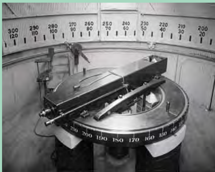
Fig. 5. Almucantar installed at Case School of Applied Science (now Case Western Reserve University) in 1900 is another instrument of precision looking very different from a traditional telescope. Like the original almucantar designed by Seth Carlo Chandler, it times rising or setting stars transiting (crossing) a fixed horizontal circle parallel to the horizon. The 6-inch telescope is the large rectangular box with an eyepiece at the left; light from a star is directed into the instrument by the angled flat mirror at its far end. Almost frictionlessly, the telescope rotates only in azimuth (instead of in altitude, like a meridian circle), as it rests on a heavy ring-shaped float in a trough of mercury. [Credit: Royal Astronomical Society, London.]
