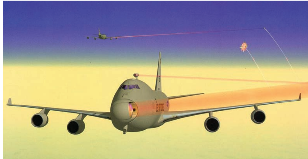
Graphic shows the experimental Boeing YAL-1 airborne laser testbed, weapons system, a megawatt-class chemical oxygen-iodine laser mounted inside a modified Boeing 747-400F. It is primarily designed as a missile-defense system to destroy tactical ballistic missiles while in boost phase.
