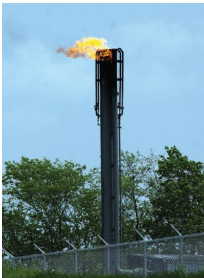
Figure 2: Unwanted methane, a powerful greenhouse gas, is routinely flared into the atmosphere in unconventional oil fields and other facilities across the U.S. and worldwide. The irony of such wholesale waste is that methane is the very product sought and monetized by drillers elsewhere, including in Ohio and Pennsylvania. Credit: Trudy E. Bell
