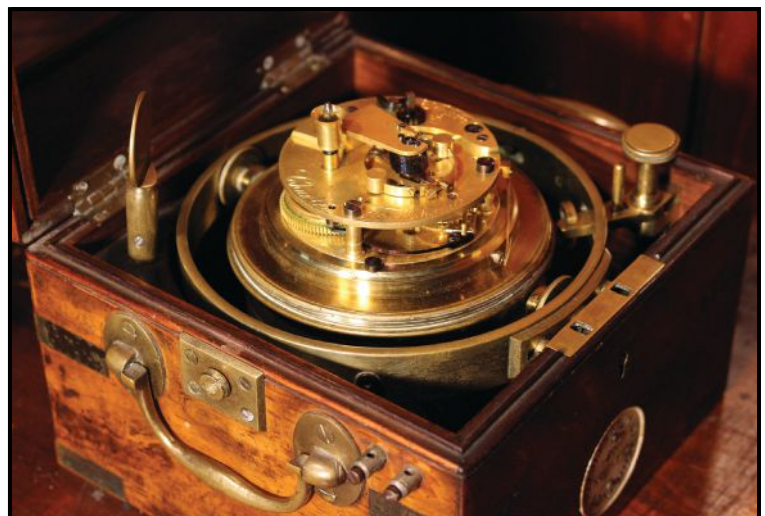
Box marine chronometer, shown face-down to display the mechanism, was made by Charles Frodsham of London between 1844-60. Parkinson & Frodsham chronometers were among the 92 chronometers used in the U.S. Coast Survey transatlantic chronometric expeditions (1849, 1850, and 1851), which sought to precisely measure the difference in longitude between the Royal Observatory, Greenwich, and the Harvard College Observatory. This chronometer, from the Ladd Observatory collection at Brown University, was later modified by Wm. Bond & Son of Boston to be used with the telegraph). Credit: Wikimedia Commons
