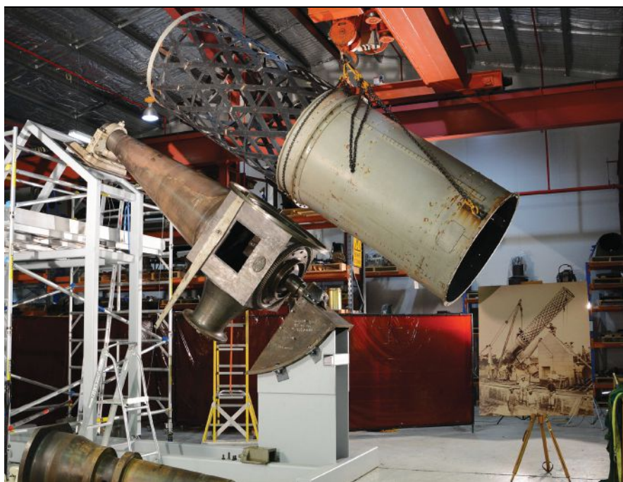
ABOVE: The Great Melbourne Telescope was assembled in Australia in early 1869; then, its protective house with a roll-off roof was put up around it. The lower third of the GMT's tube was boiler plate (wrought-iron plate of the standard used for manufacturing steam boilers) while the upper two-thirds was a cylindrical lattice of riveted iron strips. Image: Museums Victoria. BELOW: Trial reassembly of the GMT was far enough along for photos to be taken in late 2014 to aid in fundraising for the restoration project. All five of the restored pieces from Mount Stromlo are shown: cube, upper cone, bell housing, and quadrant on the supporting pier; the declination axle is lying in the foreground (partially cropped out at the bottom of the photo). Photo: John Robinson.
