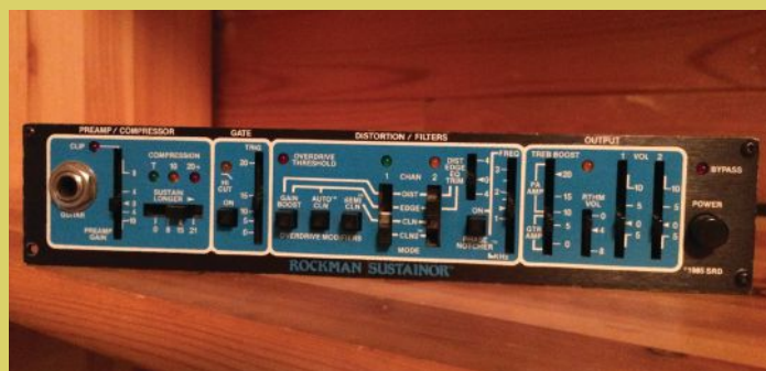
Scholz’s Rockman, the first amplifier capable of reproducing the distortion of stage speakers in the musicians’ headphones.
