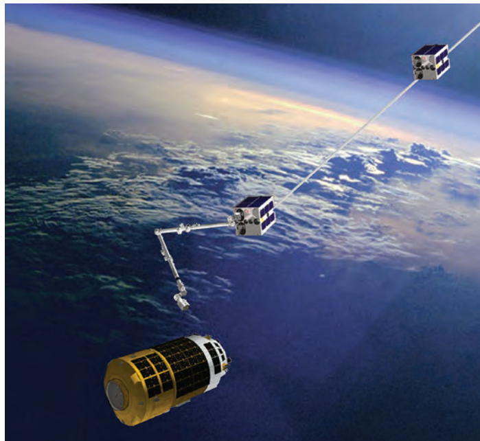
Figure 5. Most debris objects could be captured in nets, but some require a grapple device such as shown here. Devices like this have been developed and tested by NASA, DARPA, and the Naval Research Laboratory. (Canadian Space Agency, NASA, and wykesweb.com images)
