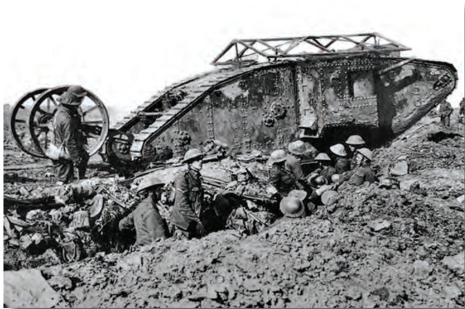
An early British Mark I “male” tank, named C-15, near Thiepval, 25 September 1916. It was probably in reserve during the Battle of the Somme. The tank is fitted with the wire “grenade shield” and steering tail, both features discarded in subsequent models. Photo: Imperial War Museum
