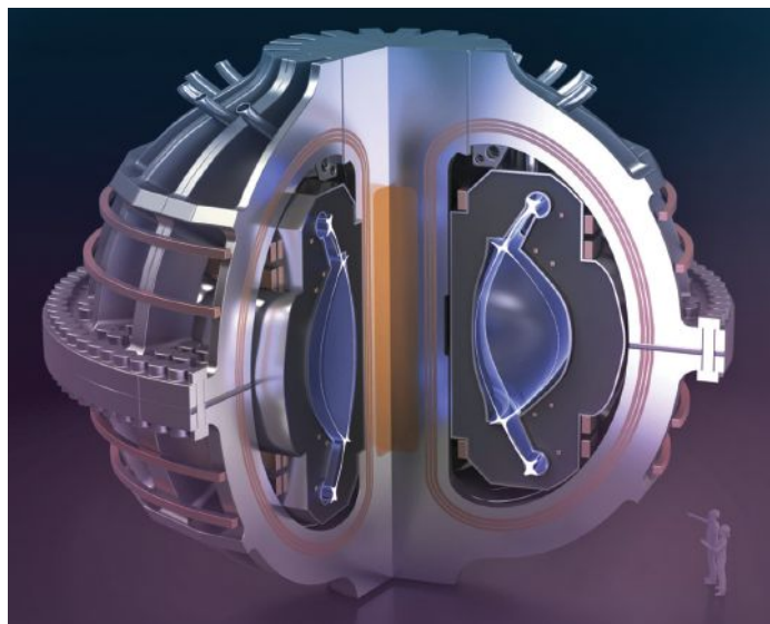
An illustration of SPARC, a compact, high-field tokamak now under construction by a joint Commonwealth Fusion Systems-MIT. Roughly the size of today's experimental tokamaks, it is designed to generate up to 100 MW of plasma energy for 10 seconds. Credit: T. Henderson, MIT.
