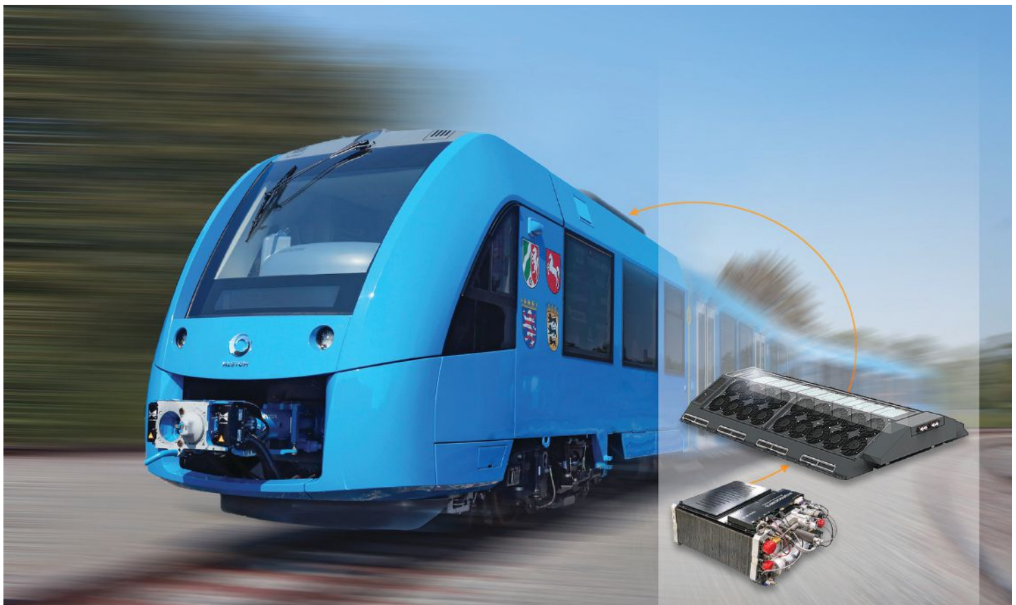
Alstom's Coradia iLint, a hydrail running up to 140km/hr (87mph), is tested and ready to roll in Germany by late 2017.
