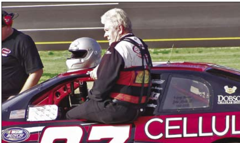
Figure 3. “Stock” cars originally had their doors welded shut for safety. The body of today’s stock cars (above) are fabricated from a single piece—completely eliminating the doors.
