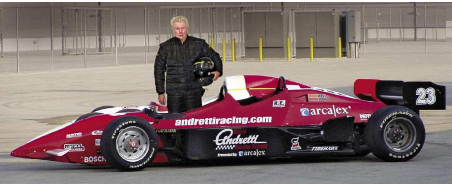
Figure 1. This “Indy” car (above) has a substitute motor that produces only 600 hp (roughly 75 percent of normal). This instructor model has been lengthened so that a passenger seat could be added.
