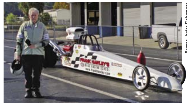
Figure 2. A gas dragster (above) boasts 700 hp on a non-supercharged 4-bbl carburetor and gasoline. The engine is available directly from GM.
