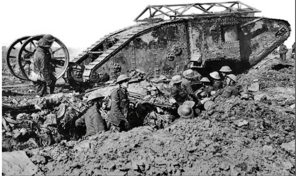
An early British Mark I “male” tank, named C-15, near Thiepval, 25 September 1916. It was probably in reserve during the Battle of the Somme. The tank is fitted with the wire “grenade shield” and steering tail, both features discarded in subsequent models. Photo: Imperial War Museum
