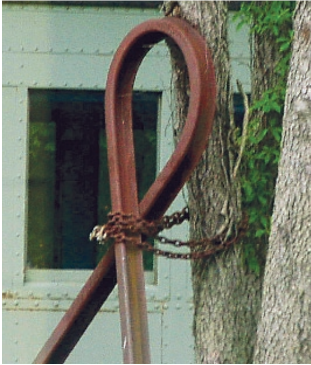
BOW-TIE: a train rail heated and bent into a shape that made it unfixable. Essex Steam Train, CT
